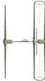
2 element with 30/40 dipole, 6m passive options
