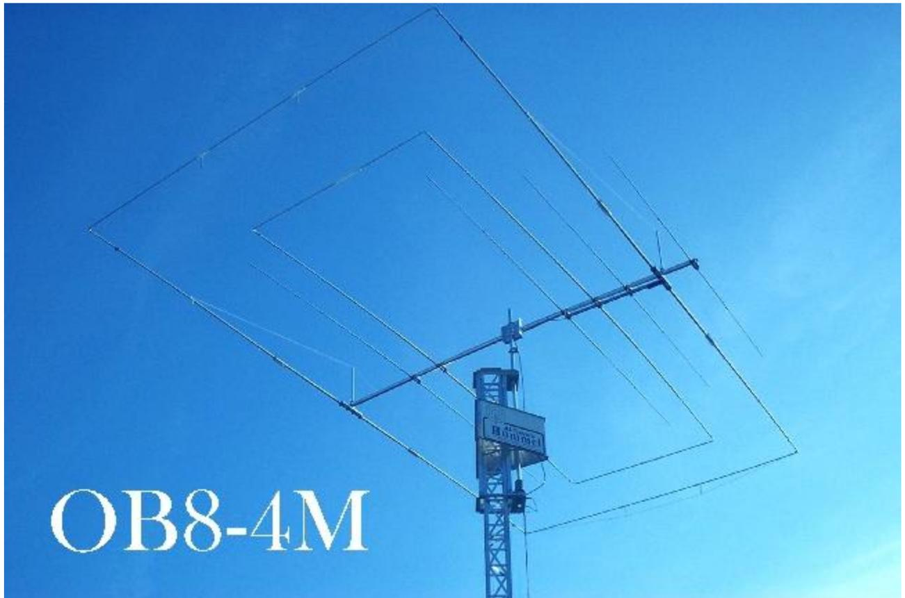
**The OB8-4M is an extremely effective, compact and innovative Yagi for the classical four bands 40, 20, 15 and 10m. It is the first trapless Yagi for this frequency spectrum in the world with a single 50 Ohm coaxial feed and with two powerful Moxon Rectangles integrated in its design to improve performance. A mechanically brilliant power house without compromise, the next level of antenna performance!**
