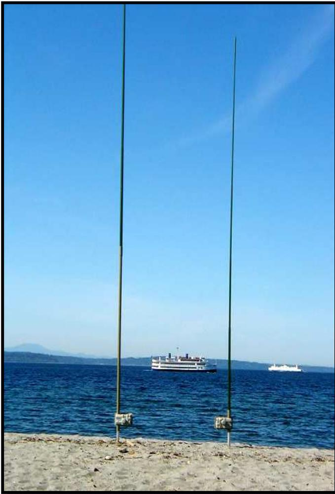
**No traps, coils, capacitors or linear loading of any kind**
